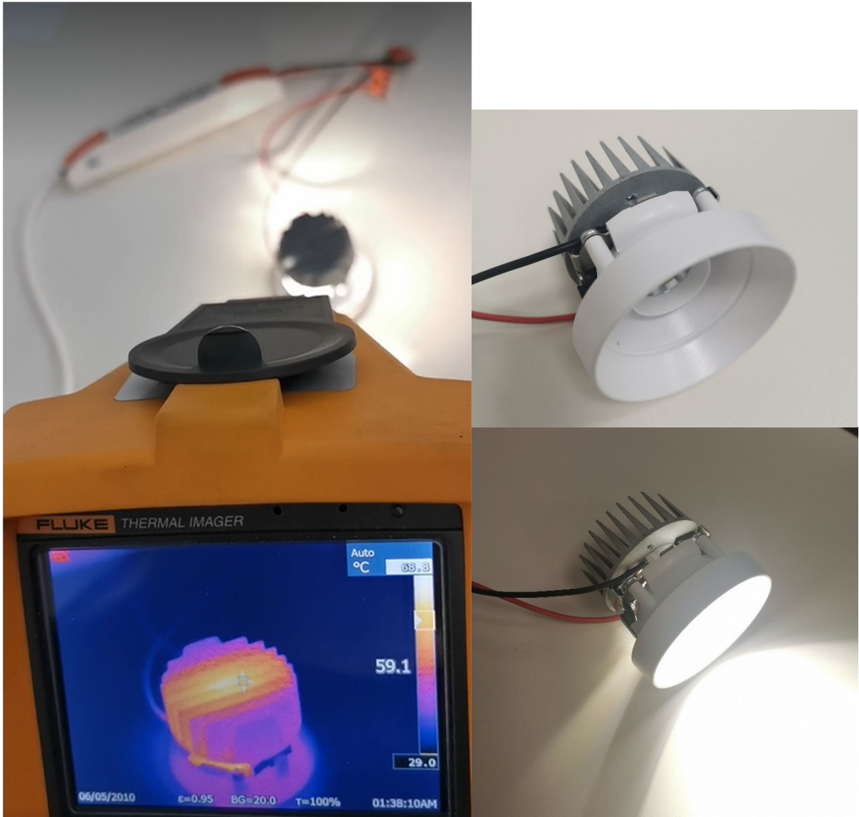
Figure 3: Intra lighting demonstrator tested with thermal camera
