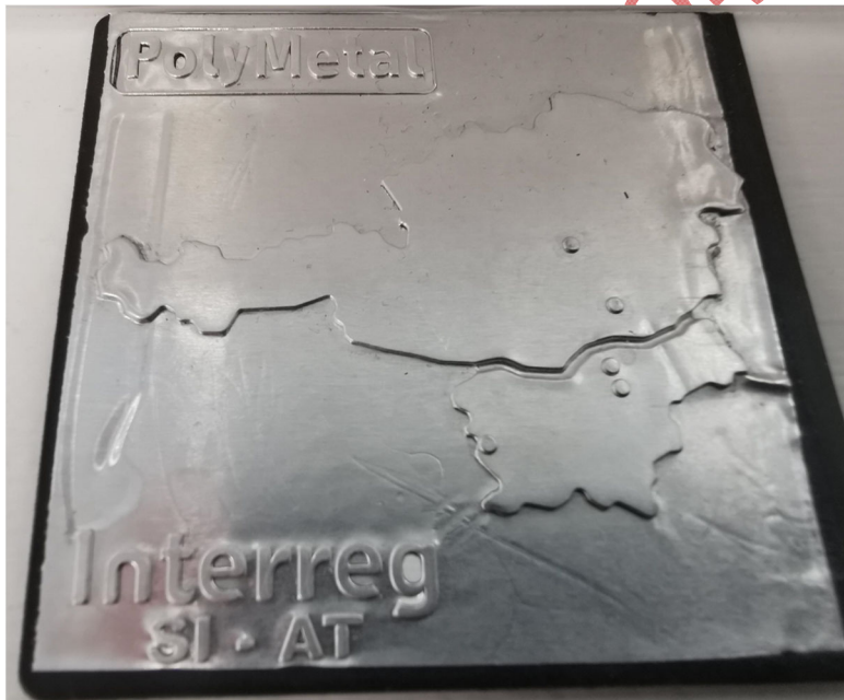
Figure 6: Produced samples from the prototype tool (composite with high thermal conductivity – top, IML technology – bottom)
