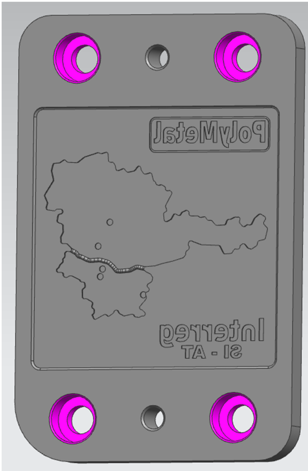
Figure 5: Prototype tool inserts with different surface roughnesses and with PolyMetal & Interreg SI-AT logos and SI-AT maps – 3D drawing
