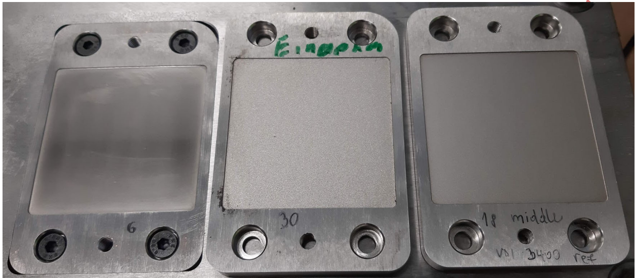
Figure 1: Prototype tool inserts with different surface roughnesses
