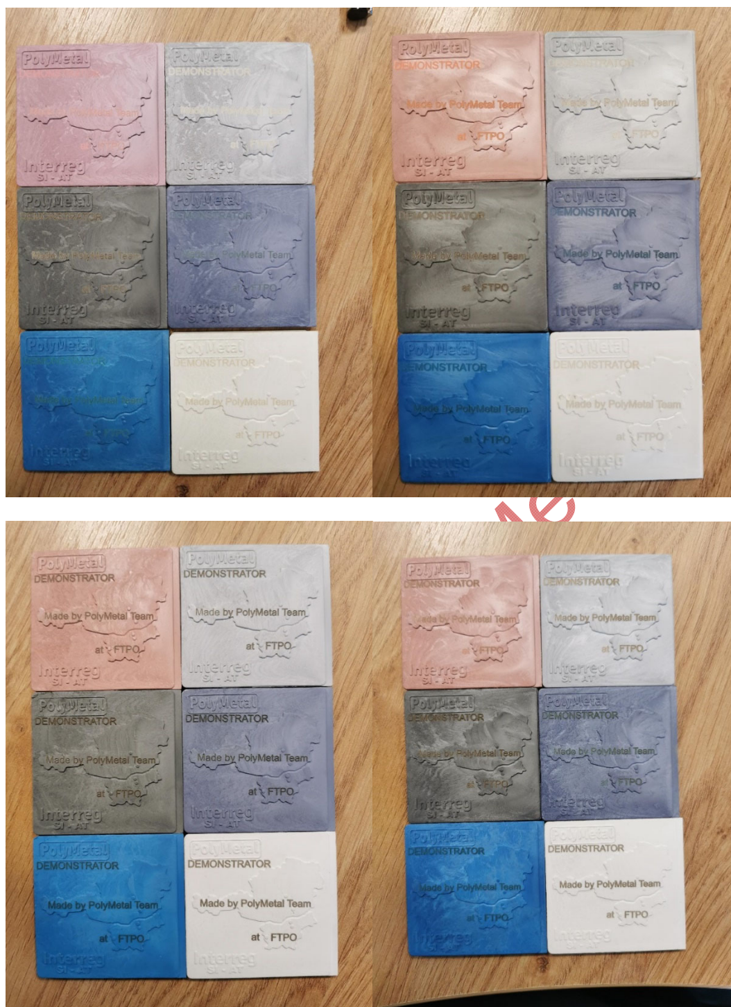
Figure 4: Produced samples of the direct injection moulding technology with the composites with high thermal conductivity and addition of metallic Master Batches (from top to bottom and left to right: PA 6, PP, ABS, PS, PC) in the prototype tool
