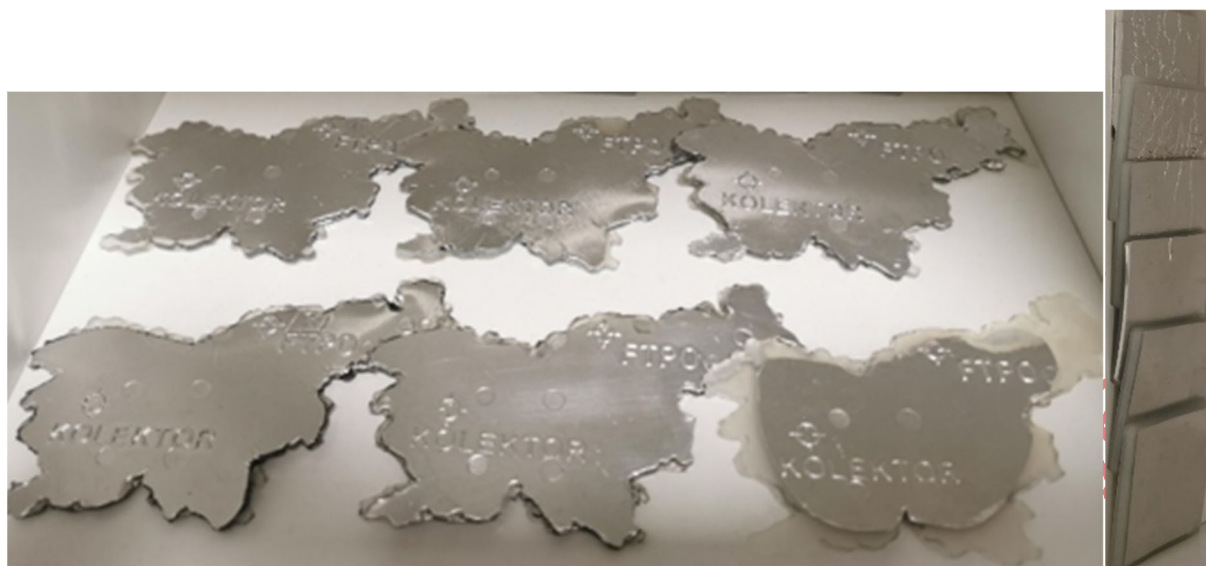
Figure 5: Produced samples of the IML technology with different thicknesses of Al foils
