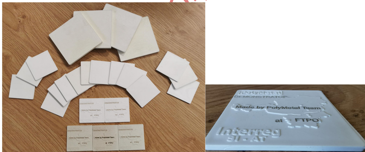
Figure 3: Produced samples of the direct injection moulding technology with the composites with high thermal conductivity
