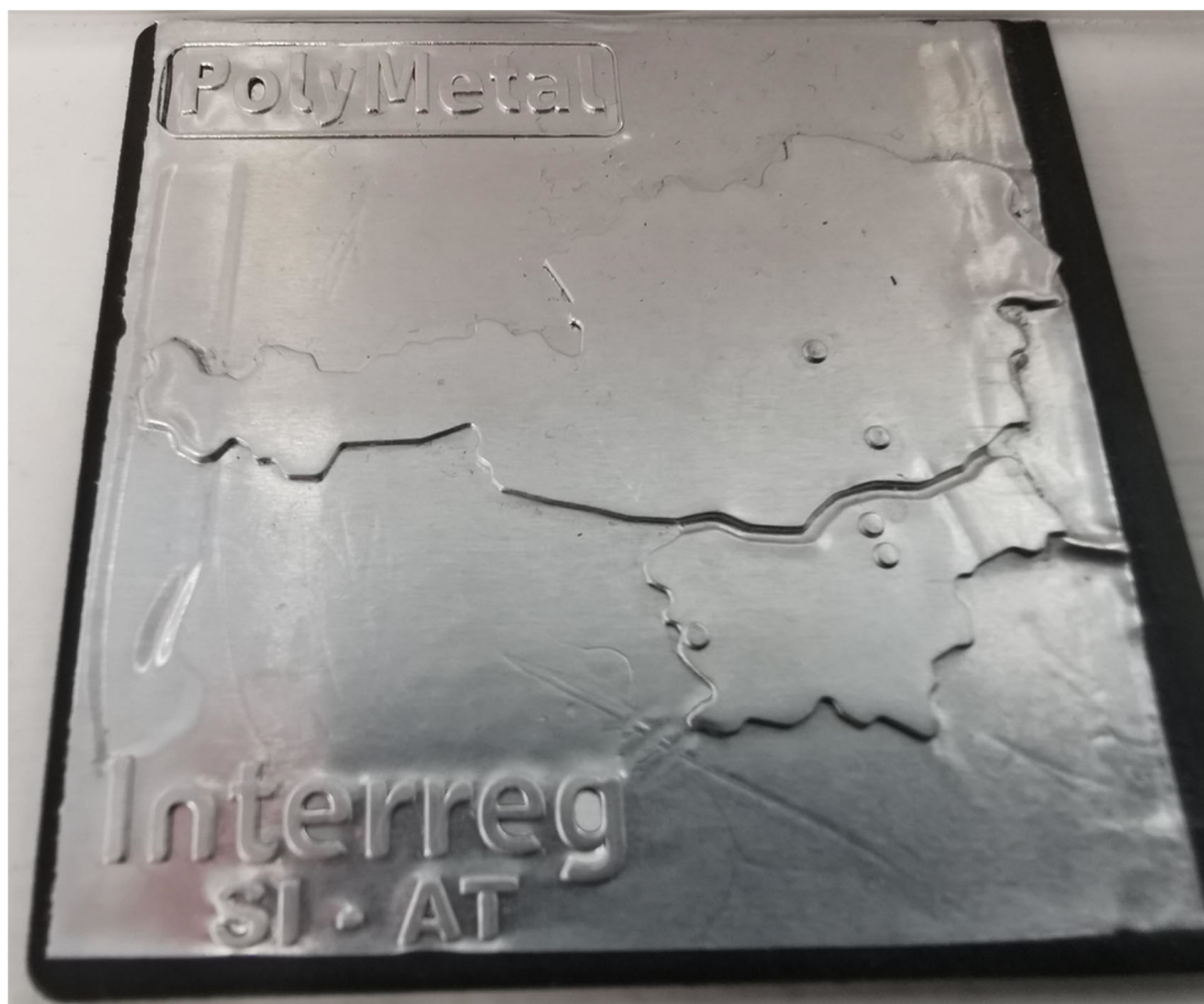
Figure 8: Produced samples of the IML technology in the prototype tool
